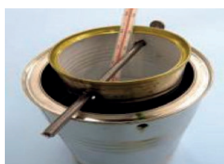
Figure 5.4: Measuring water temperature in the calorimetre.
