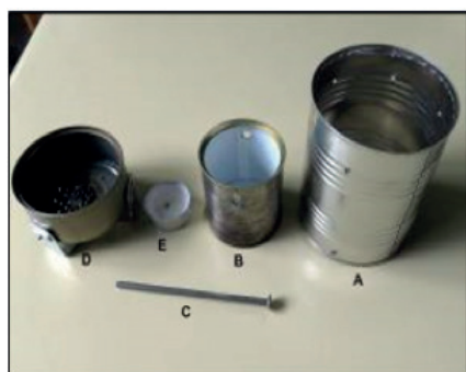
Figure 5.2: Materials to make the calorimeter.
