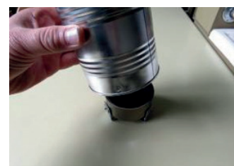
Figure 5.3 B: Assembling the calorimetre.
