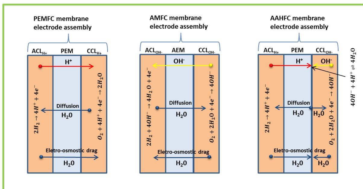
**Fig. 1** Schematic of PEMFC, AMFC and AAHFC
