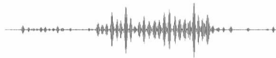
Figure 4: Example of a dance rhythm. This figure shows the pulse patterns generated by the wings that can be measured as alternating electromagnetic fields. The highly modulated part, here approx. 1 sec long, is the actual waggle run and encodes the distance to the feeding source. The breaks show the concentricity/circular run to the next starting position. The consecutive waggle runs are danced alternately rightwards and leftwards, following a figure-of-eight shape. The direction of the dance during waggling encodes the direction of the food source in relation to the position of the sun (not visible from the signal).
